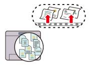
The Stored Print feature allows you to temporarily store your print data in the printer memory and output it later. You can effectively manage your time when you print confidential data or large-volume data at off-peak hours.
